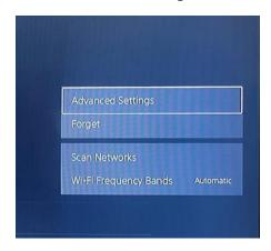
From Wifi Frequency Bands, select 5 GHz. This should cause your device to disconnect and reconnect.
